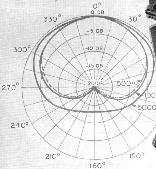
Directional characteristics of the BK-5A Microphone about the vertical axis.
