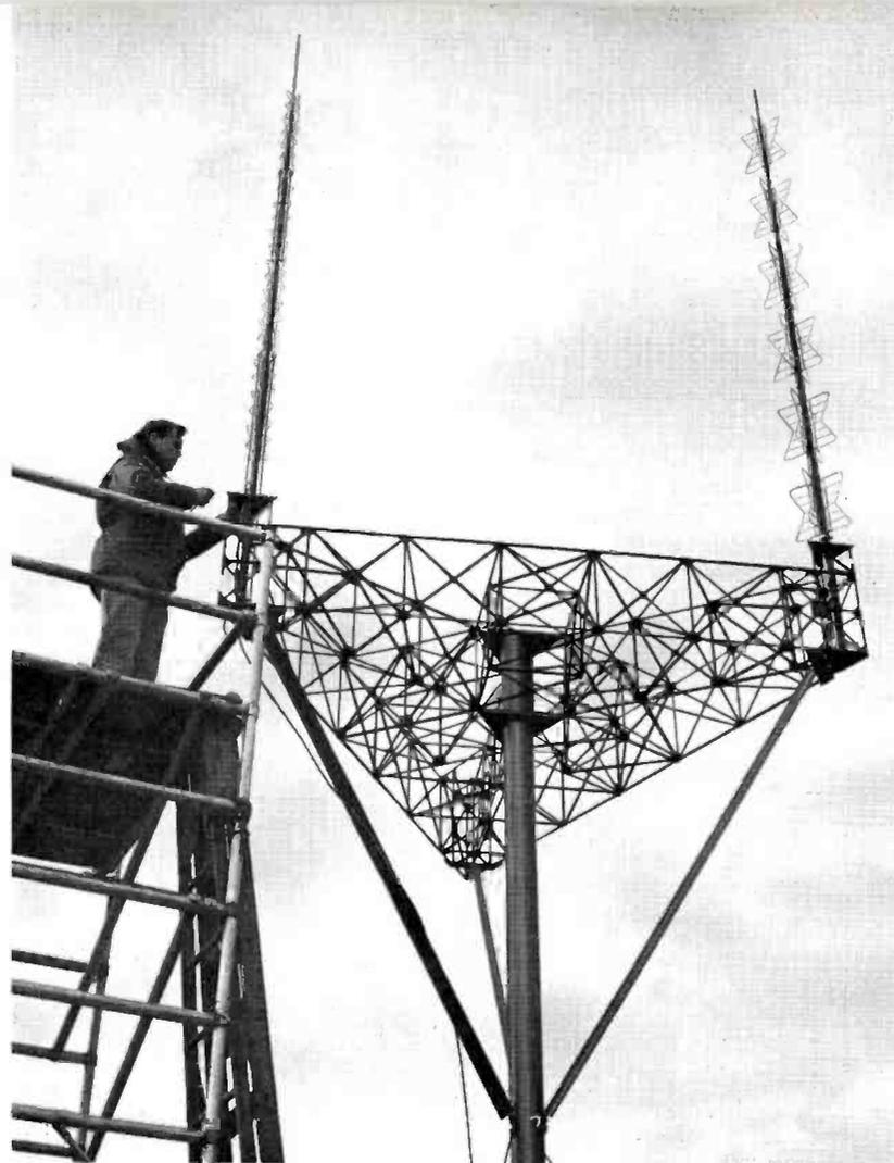
To acquire performance data on antennas mounted side-by-side in reasonably close proximity, working model antennas built to one-tenth scale and operating in the region of 500 to 1500 mc. were used. The supporting triangular platform is also a scaled replica of the completed installation.
