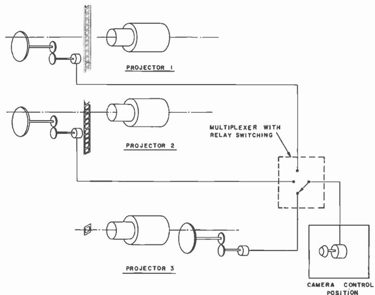
FIG. 10. Multiplexer system for varying light controls.
