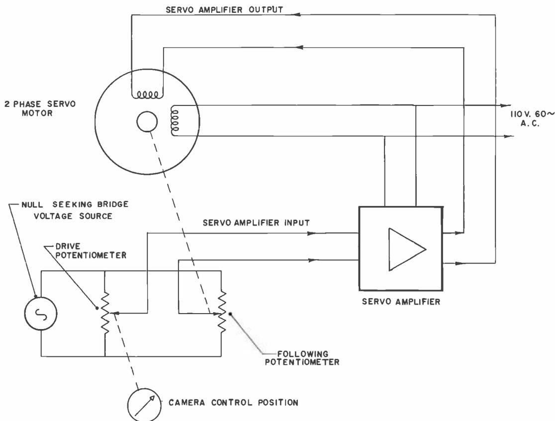
FIG. 3. Bridge circuit which drives the filter wedge.
