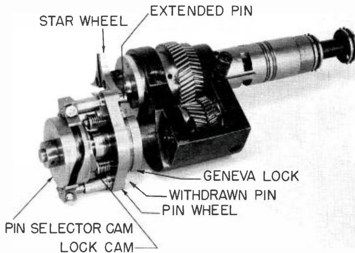
FIG. 6. Overall view of complete intermittent.
