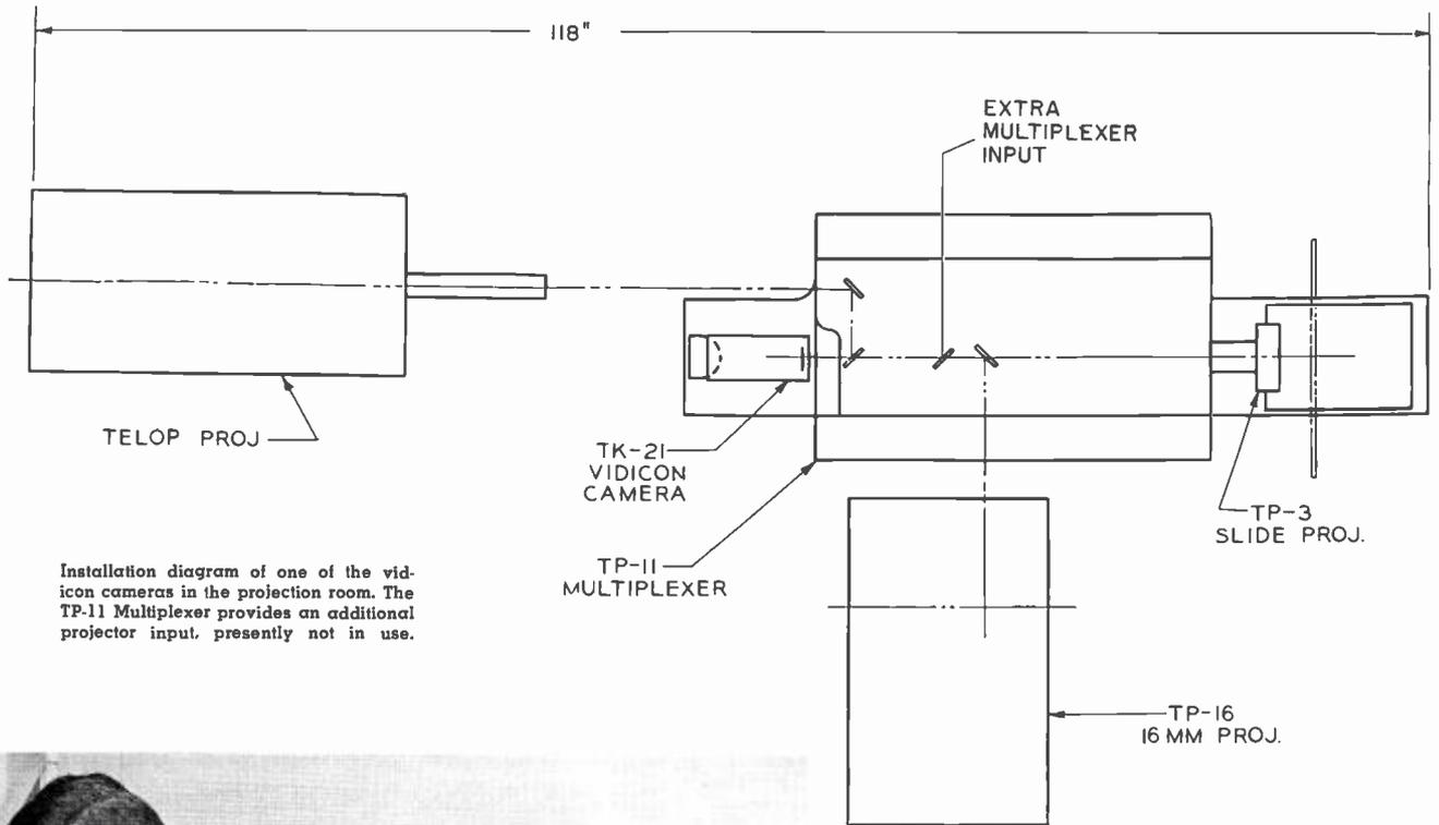
Installation diagram of one of the vidicon cameras in the projection room. The TP-11 Multiplexer provides an additional projector input, presently not in use.
