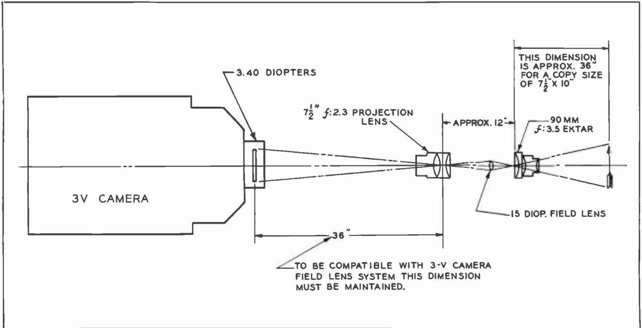
FIG. 2. Optical system showing lens arrangement for live commercial pickup. The Ektar lens is identical with those used on RCA image-orthicon cameras.
