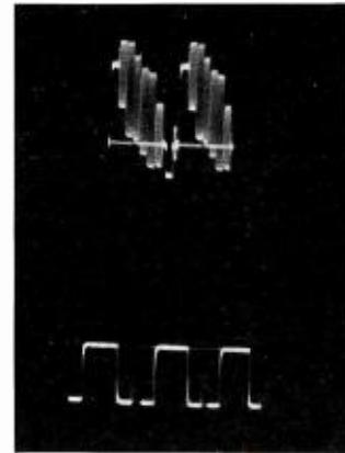
FIG. 15. Above: Colorplexer output signal for a color bar test pattern displayed at half-horizontal frequencies. Below: Typical display showing calibrating square wave with electronic calibration lines superimposed in the background.
