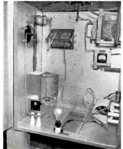
FIG. 15. Interior of LTU. 100 watt bulb keeps down dampness—provides light for reading meter through the door porthole.
