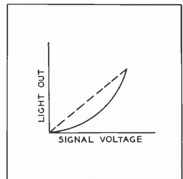
FIG. 8. Transfer curve of an average kinescope.
