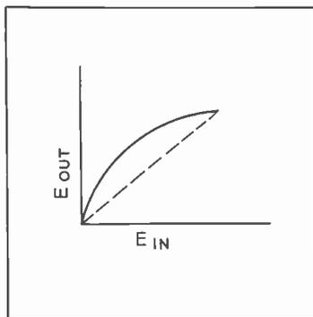
FIG. 9. Transfer curve of the television camera system.
