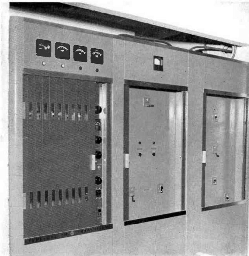
FIG. 4. RCA BTA-1M 1 kilowatt transmitter, left, with power dividing and branching equipment mounted in two matching right wing phasing cabinets. Day/night switching facilities are in cabinet directly to right of BTA-1M.
