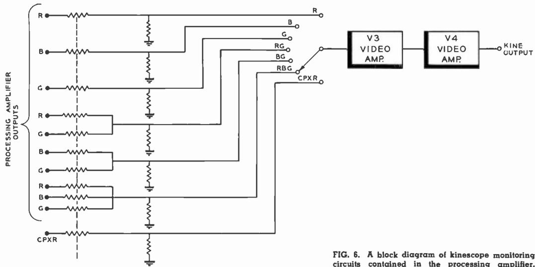
FIG. 6. A block diagram of kinescope monitoring circuits contained in the processing amplifier.
