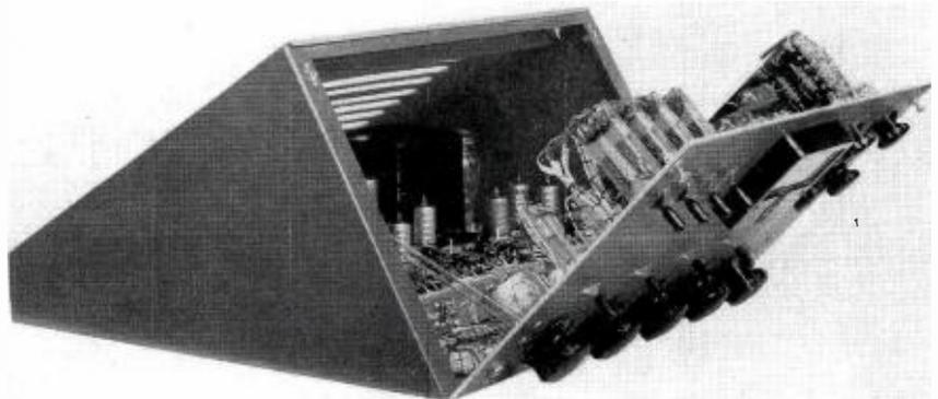
FIG. 3. View showing BC-5A interior by opening front panel. Printed wiring boards are mounted on horizontal chassis. Another is visible at upper right corner inside front panel.
