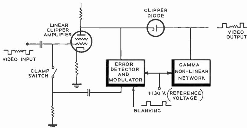
FIG. 7. A block diagram of feedback clamp circuit.
