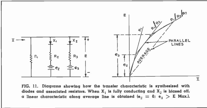
FIG. 11. Diagrams showing how the transfer characteristic is synthesized with diodes and associated resistors. When  $X_1$  is fully conducting and  $X_2$  is biased off, a linear characteristic along average line is obtained ( $e_2 = 0$ ;  $e_3 > E$  Max.).
