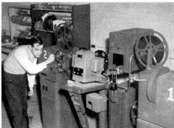
FIG. 6. The film room is equipped with two RCA 16mm TV film projectors. 35mm slide projector and RCA film camera.
