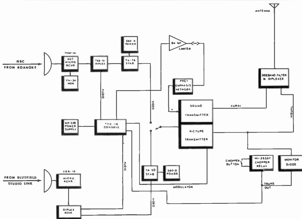
FIG. 1. Block diagram showing studio and transmitter equipment with connecting microwave link.
