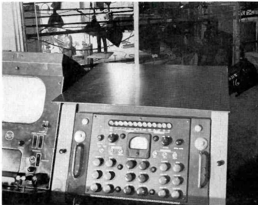
FIG. 6. Color TV control room showing from left to right—the RCA 21-inch color receiver, Camera Control Panel, Processing Amplifier and the associated rack and test equipment.
