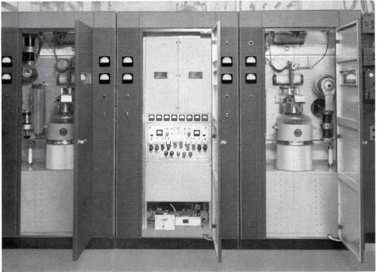
Part of new RCA type BTA-50G AM transmitter just prior to shipment to station WINS. Three of the four cubicles are shown—the two final power amplifier cubicles on either side of the exciter unit.
