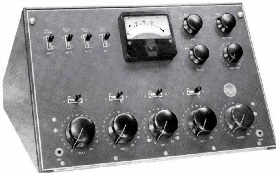
FIG. 1. The BC-5A Audio Console. Modular construction, nine inputs, three preamps. Has talk-back and program cue to remotes, program and audition facilities. Uses etched-wiring amplifiers.
