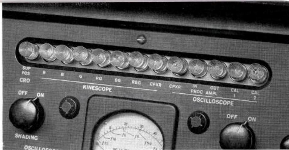
FIG. 13. Close-up of the push buttons of the electronic switcher.
