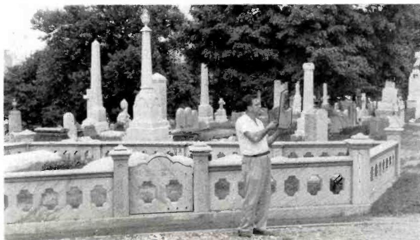
FIG. 18. This and the above photos show monitoring point locations selected to monitor the operation of the two directional antenna systems. Chief Engineer Frank Unterberger uses RCA WX2C Field Intensity Meter.
