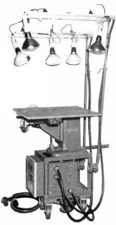
Mounted on the base of the milling machine is a lighting switch panel. This serves to distribute power to the three adjustable lighting booms, the light box, the turntable and two accessory outlets. The lighting booms were constructed from discarded music stands and are adjustable both in elevation and angular position. Plugmould outlets are fastened to the boom, providing ac facilities along the length of the boom. Clamp-on adjustable sockets serve as the spot and flood light holders.
