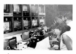
FIG. 2. Main studio control room monitor table, showing the various picture sources handled during a representative part of a convention day.
