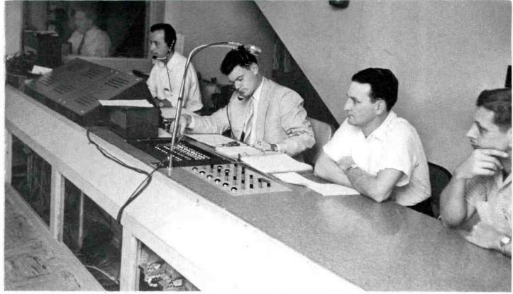
FIG. 10. Studio "A" production control room, larger of two control rooms. Elevated three feet to effect good visibility. Twenty-foot control desk extends full width of room. Equipment looking from foreground consists of: lighting remote control, intercom control. TS-20A Video switcher. TG-15A special effects, BCM-IA mixer, BC-2B consolette, tape recorder and play back.
