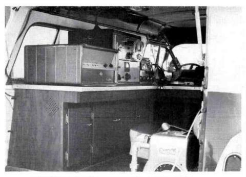
FIG. 4. This 500-watt gasoline generator mounted at the right rear of the mobile truck supplies enough power to operate all of the unit's equipment.
