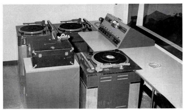
FIG. 8. Availability of a third turntable in each control room is responsible for much of the smoothness of WMCA operations. Control room for Studio "A" with three Type 70-D turntables is shown.
