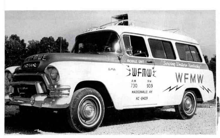
FIG. 1. Mobile unit remotes are relayed to station via 450-mc broadcast relay band.
