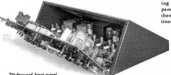
Tilt-forward front panel permits quick accessibility to mixer pads and spring contacts; makes maintenance easy. Ask your RCA Broadcast Sales Representative for detailed information
