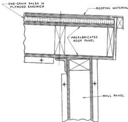
FIG. 15. Cross section of the transmitter house roof showing construction details.
