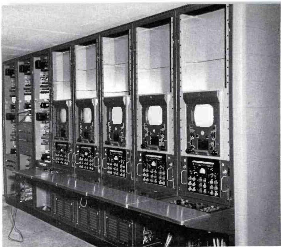
FIG. 15. Camera control room in AFIP building handles three studio cameras, the autopsy camera, and the film camera (also inputs from other areas to which studio cameras may be moved).
