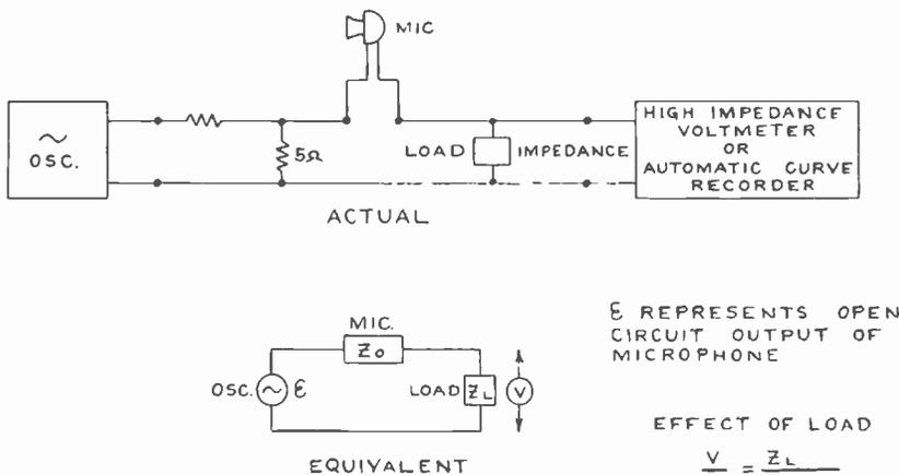
FIG. 4. Circuit used to measure the effect of load upon frequency response of a microphone. The actual circuit is shown at the top and the equivalent circuit at the bottom.
