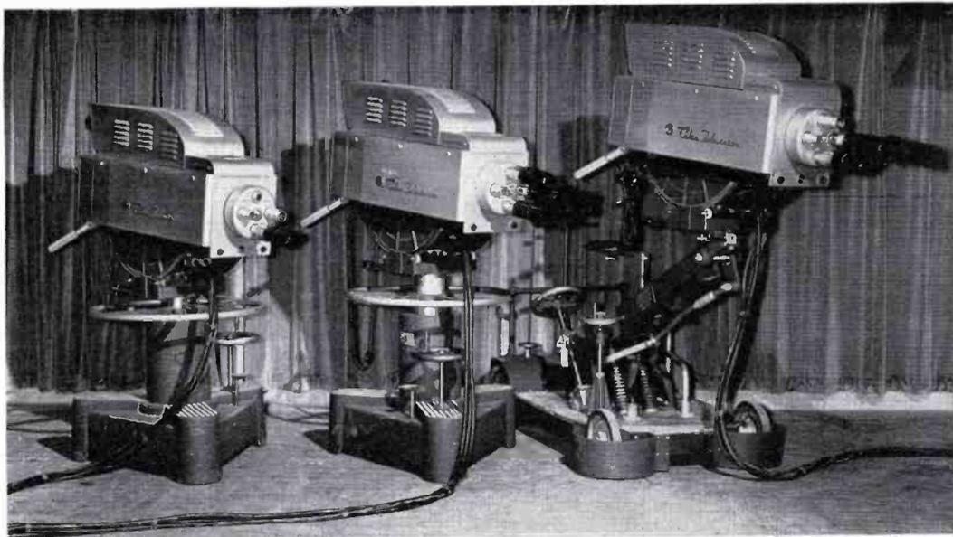
FIG. 7. Facilities in the main studio at AFIP include these three TK-41 Color TV Cameras.
