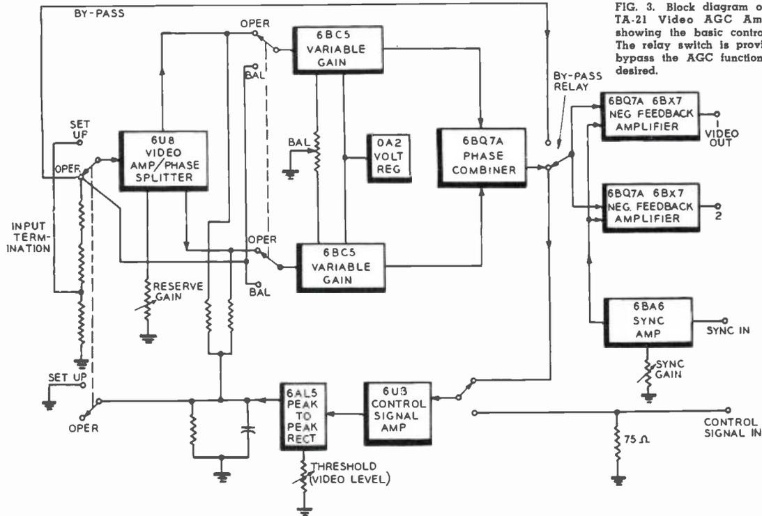
FIG. 3. Block diagram of Type TA-21 Video AGC Amplifier showing the basic control loop. The relay switch is provided to bypass the AGC function when desired.
