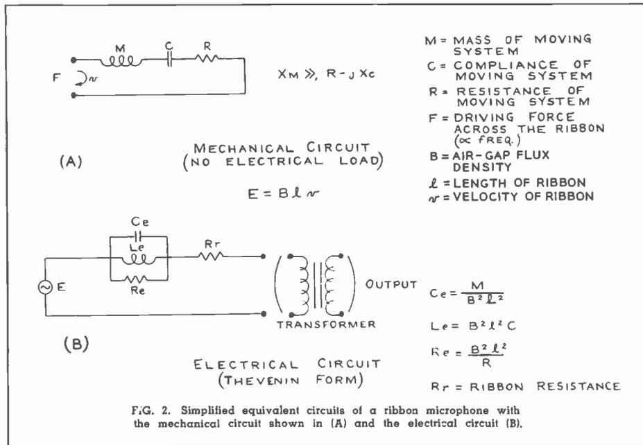
FIG. 2. Simplified equivalent circuits of a ribbon microphone with the mechanical circuit shown in (A) and the electrical circuit (B).
