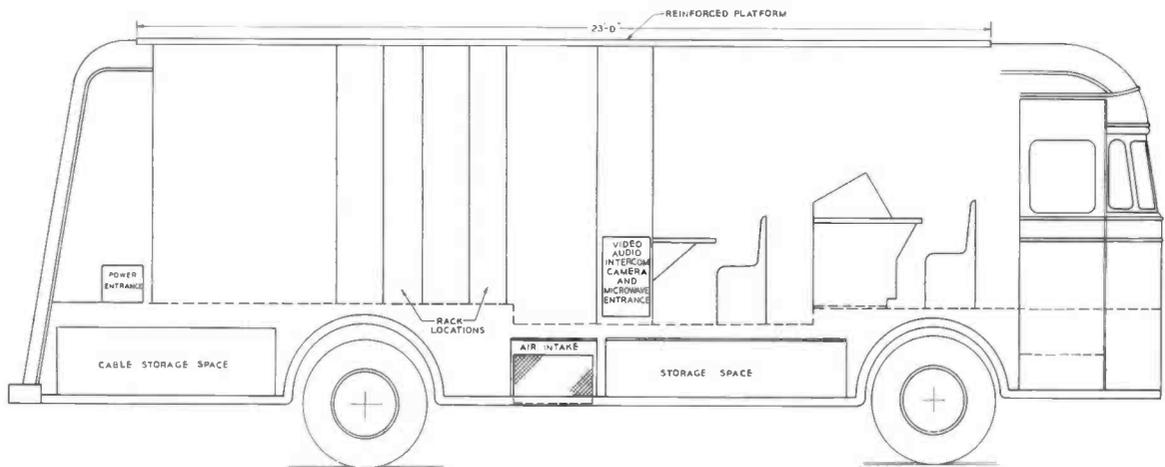
FIG. 3. Side elevation view of mobile control room.
