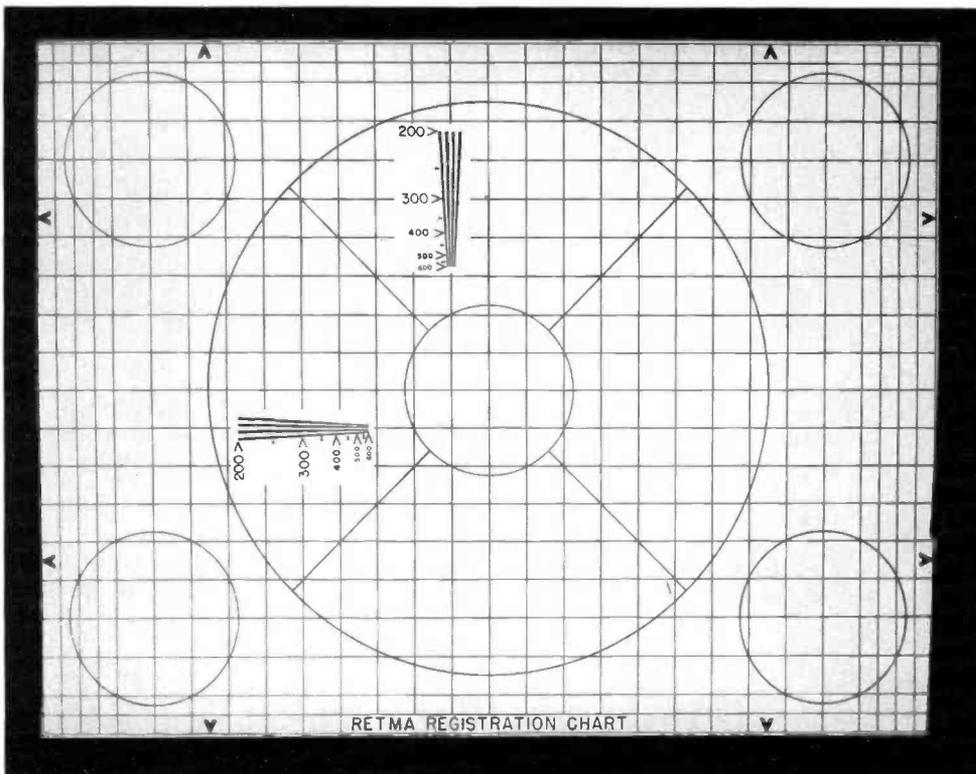
FIG. 2. Specifications for 8 by 10 inch Transparency of RETMA Registration Chart can easily be met by any commercial photographic house.
