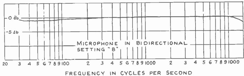
FIG. 5. Frequency response relative to no load with the microphone of Fig. 3 loaded by the preamplifier shown in Fig. 1.
