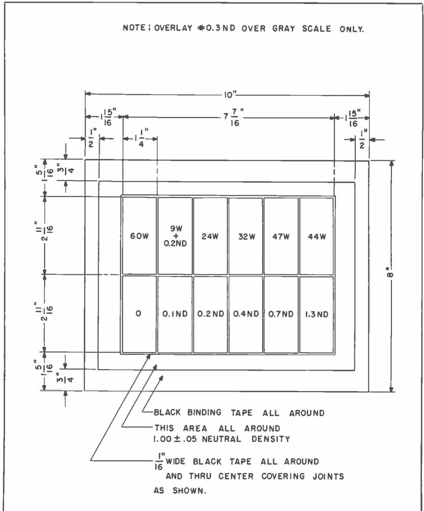
FIG. 7. NBC Color Bar Transparency is made up of pieces of Eastman Kodak Wratten filters.
