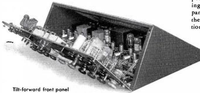
Tilt-forward front panel permits quick accessibility to mixer pads and spring contacts; makes maintenance easy.
