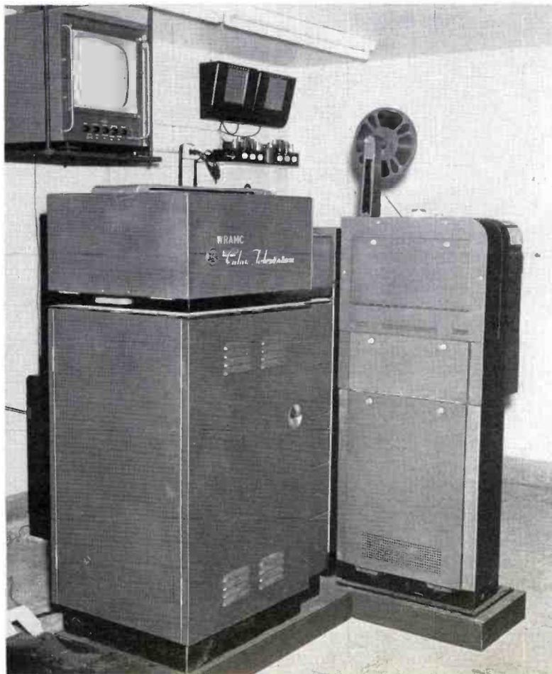
FIG. 14. The Three-Vidicon Color Film Camera is employed in film area in conjunction with 16mm motion-picture projector, 35mm and 3¼ x 4-inch slide projectors. Color as well as monochrome may be projected. These films and slides can be integrated into teaching demonstrations from any of the three buildings whenever needed.
