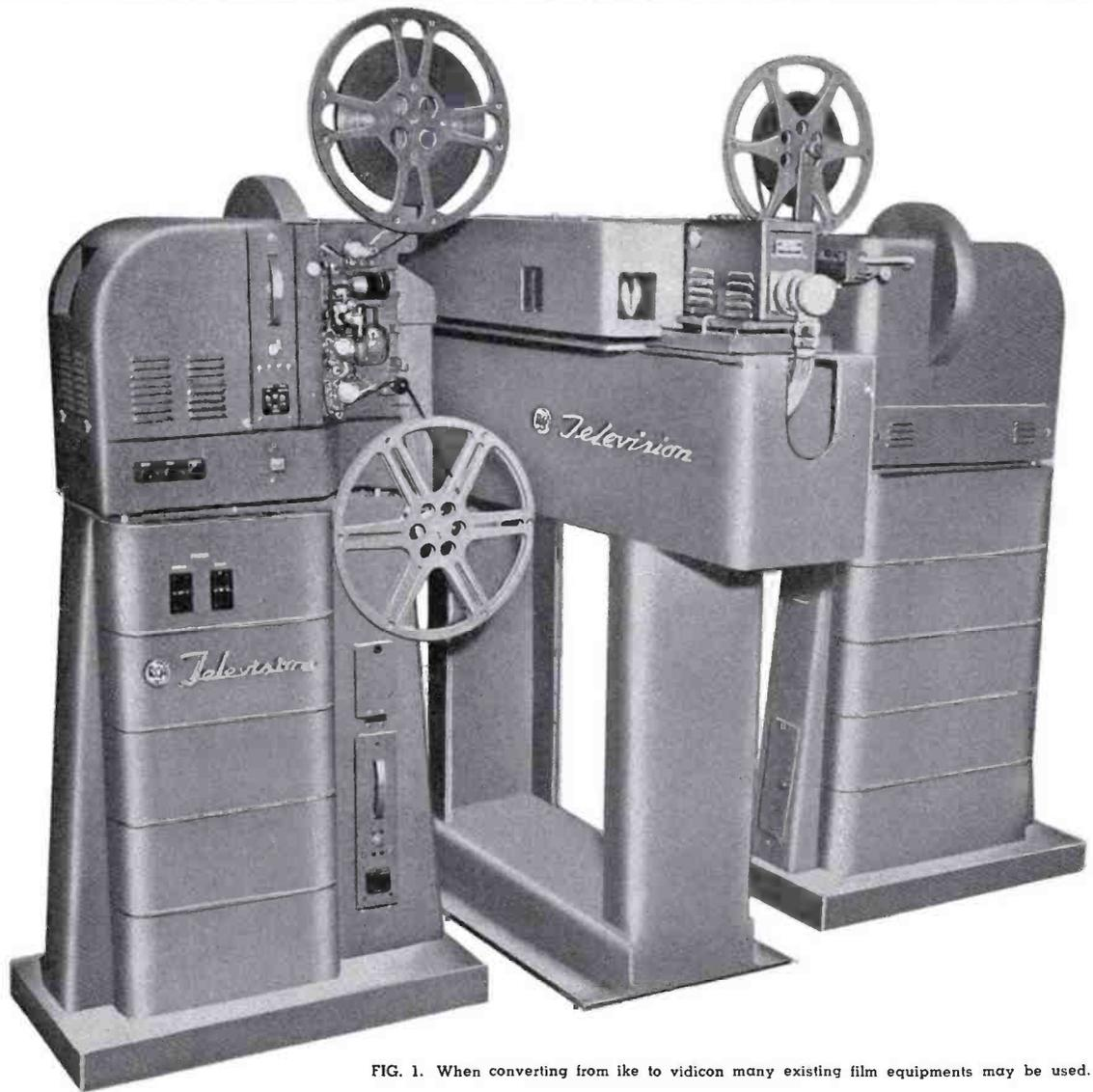
FIG. 1. When converting from ike to vidicon many existing film equipments may be used.
