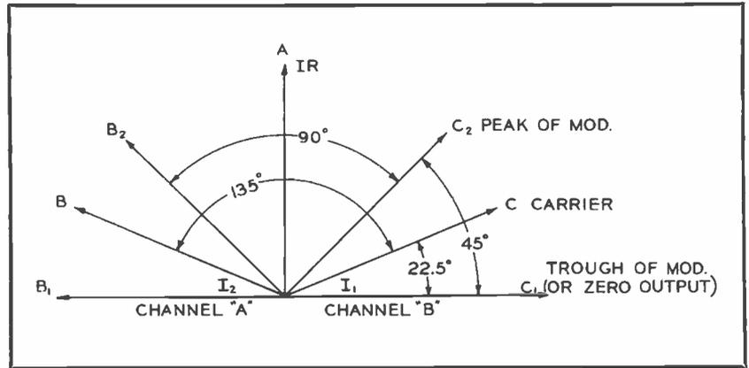
FIG. 6. Ampliphase vector diagram.
