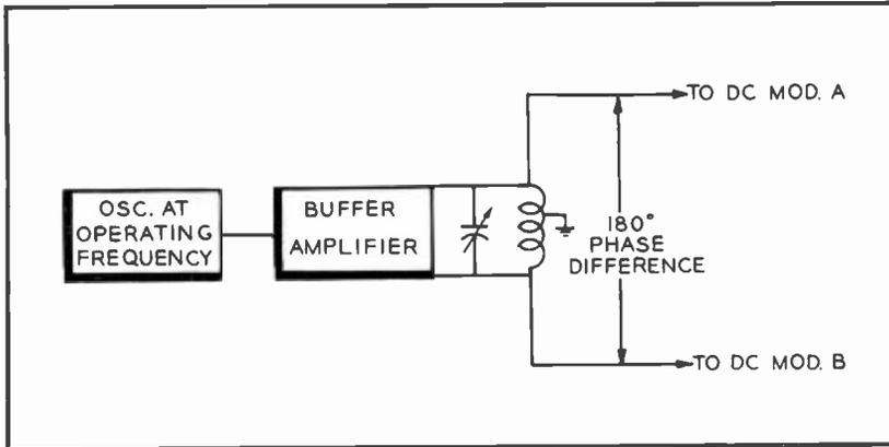
FIG. 4. Exciter-Modulator circuit.
