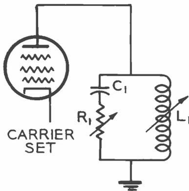
Values of L and C chosen so change in R does not change load impedance, only phase.
