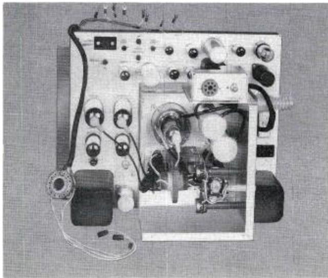
FIG. 13. Deflection and high-voltage chassis.
