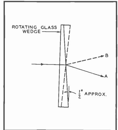
FIG. 2. Sketch showing exaggerated deviation of image resulting from use of optical orbiter.
