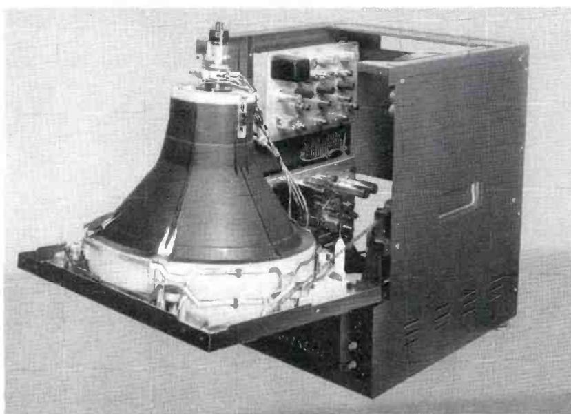
FIG. 6. Monitor front panel is readily swung down for quick removal of kinescope. ▼
