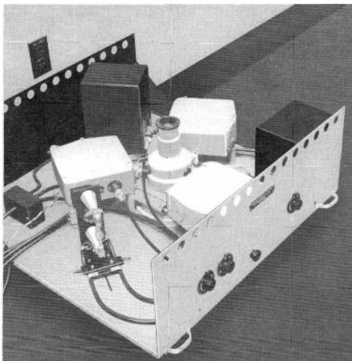
FIG. 4. Illuminating system for Ultraviolet Color-Translating Television Microscope.
