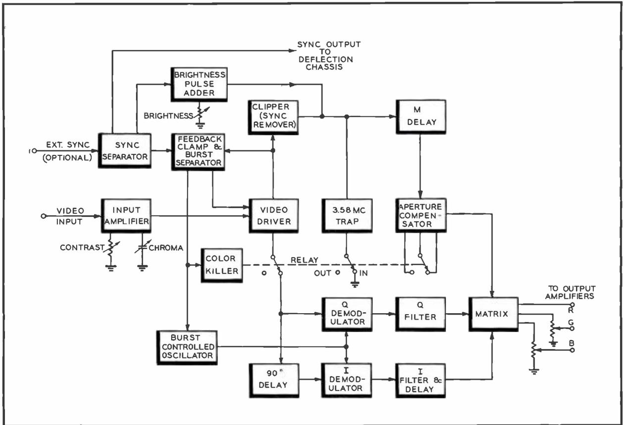
FIG. 7. Simplified block diagram of the TM-21 decoder.
