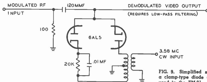
FIG. 9. Simplified schematic of a clamp-type diode demodulator used in the TM-21.
