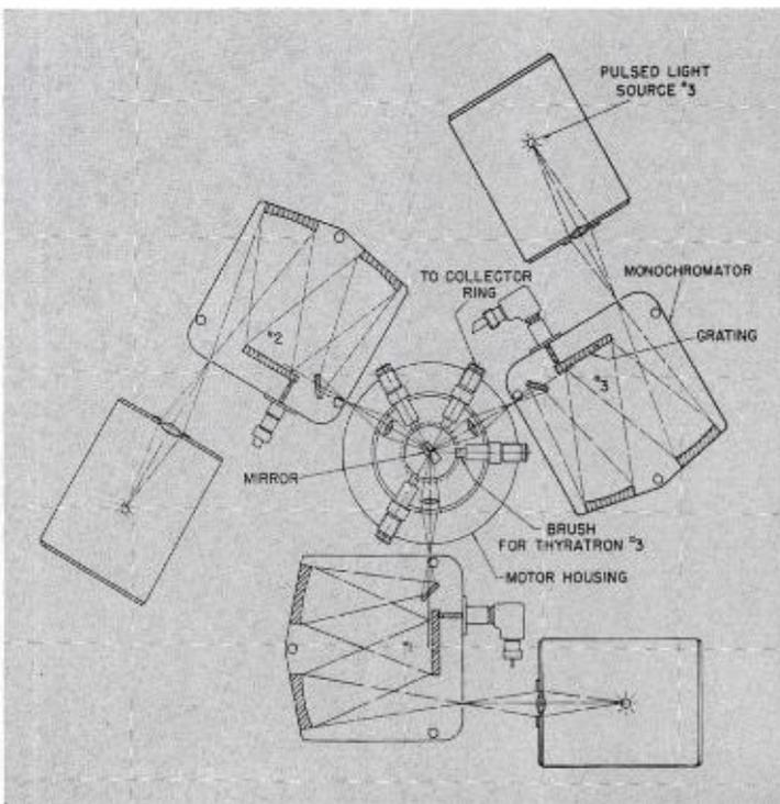
FIG. 5. Schematic diagram of illuminating system for UVCTM.
