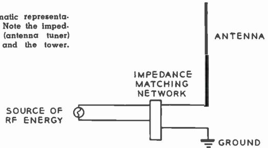
FIG. 17. A shunt-fed tower is represented here. Observe the feed point. The section of the tower between the feed point and ground offers an impedance at the operating frequency of the station.
