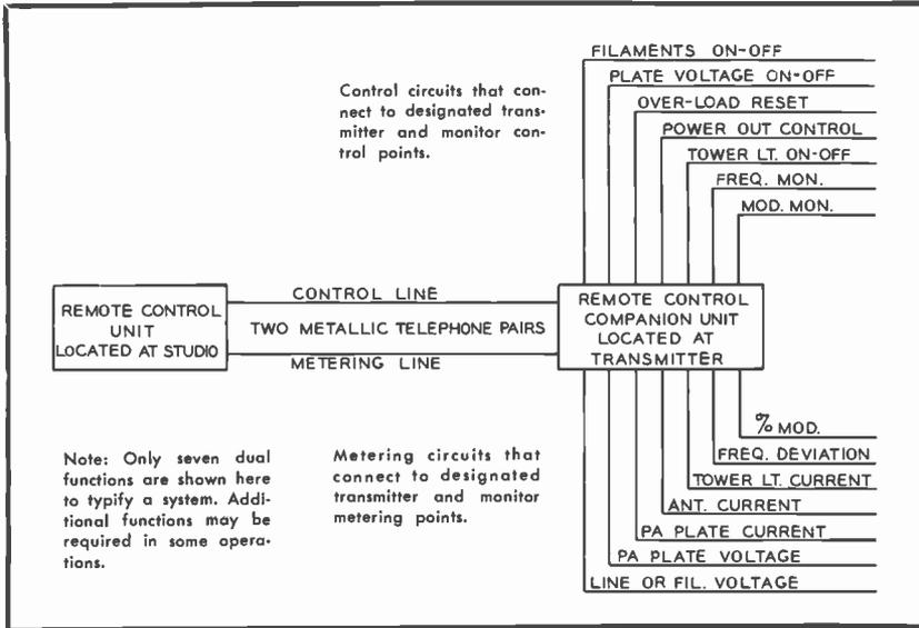
FIG. 12. Block diagram of a typical remote control system. Two telephone lines are used between the studio and transmitter. One line is for control, while the other is for metering. Additional functions may be added to the system when needed.
