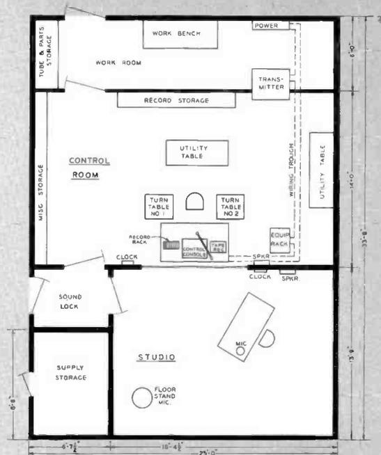
FIG. 2. Layout for Plan "B." This is similar to Plan "A" but has more facilities. It is a design for the medium-size station.
