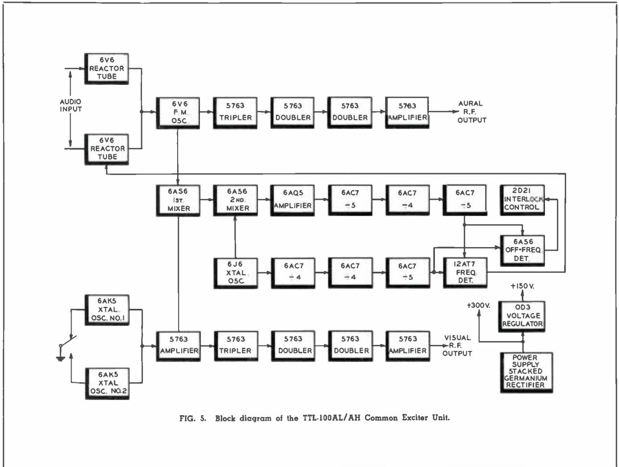
FIG. 5. Block diagram of the TTL-100AL/AH Common Exciter Unit.
