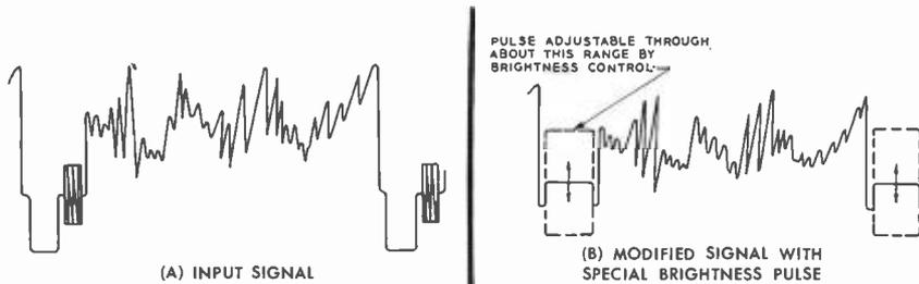
FIG. 19. Waveform sketches illustrating the operation of the BRIGHTNESS control.
