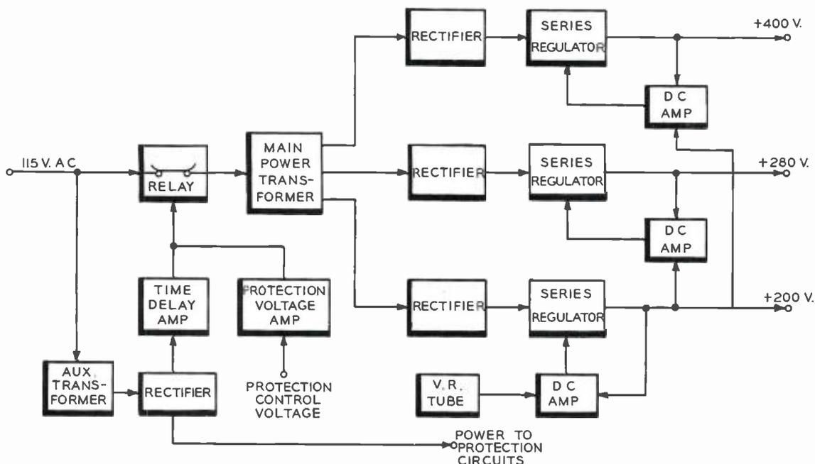
FIG. 16. Block diagram of three-in-one power supply.
