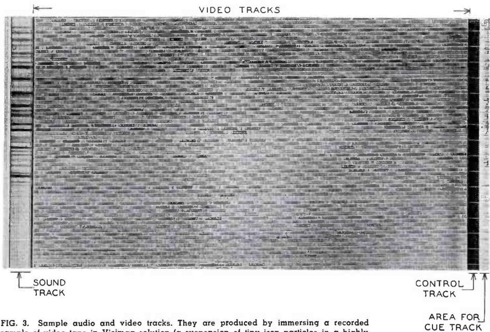
FIG. 3. Sample audio and video tracks. They are produced by immersing a recorded sample of video tape in Visimag solution (a suspension of tiny iron particles in a highly volatile liquid). The iron particles cling to the magnetic areas, and once the fluid evaporates, the magnetic pattern becomes visible. The pattern shown here was picked off the video tape onto a strip of transparent adhesive tape, then photographed and engraved.
