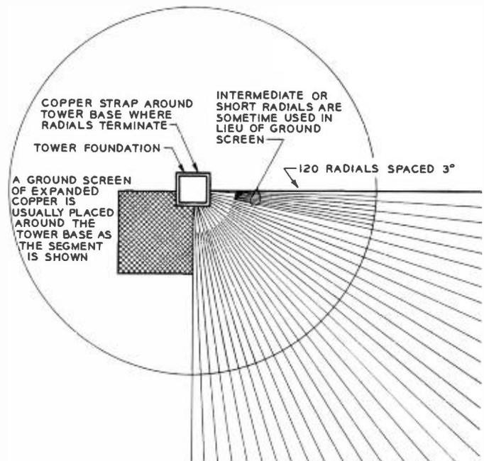
FIG. 18. Typical ground system constructed about the antenna. Radials are placed around the base of the tower to form a complete circle. A ground screen or mat is also positioned all of the way around the tower base. (Note that this drawing shows radials and the mat in only one quadrant, whereas both actually go completely around the tower.)
