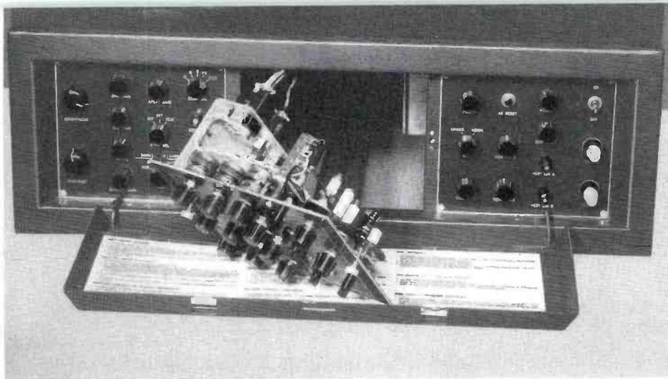
FIG. 4. Front view of the TM-21, with the convergence chassis withdrawn for easy servicing. Contained in cover is detailed procedure for kinescope set-up, including convergence.
