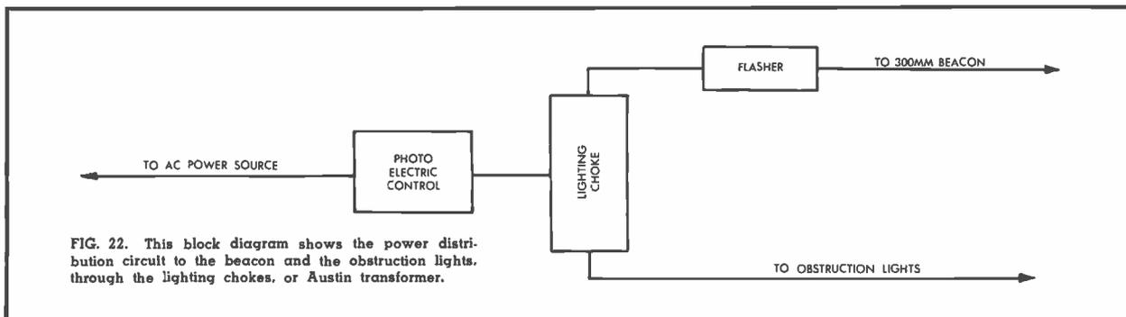
FIG. 22. This block diagram shows the power distribution circuit to the beacon and the obstruction lights, through the lighting chokes, or Austin transformer.
