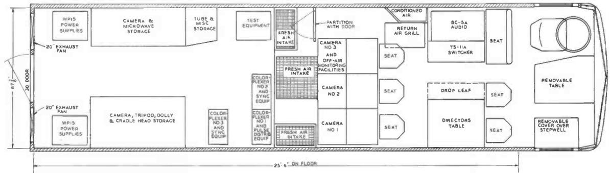
FIG. 5. Plan view of mobile control room.
