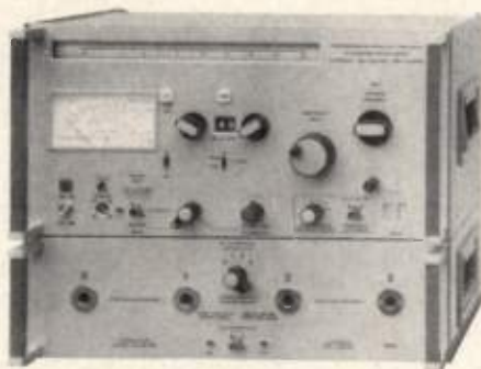
Schwarzbeck FSME 1515 Receiver and NNBM 8112 LISN. The Standard Configuration Used By The VDE, and All Over The World.
