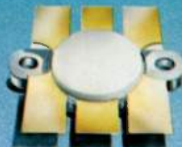
SD 1441 130 → 175 MHz – 150 W SD 1468 225 → 400 MHz – 70 W SD 1499 450 → 512 MHz – 65 W
