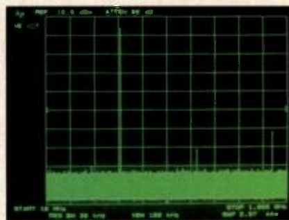
Frequency spectrum of Andersen Model SO-314-600-V Oscillator over 0 to 1 GHz range. Fundamental frequency is 314 MHz. Second harmonic is -65\text{dBc} , third harmonic is -55\text{dBc} . Spurious responses are essentially nonexistent.
