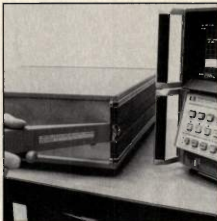
Figure 4. Searching for electromagnetic energy leaks at seams of an enclosure.
