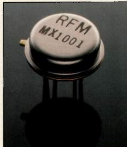
The AM Microtransmitter from RF Monolithics puts a SAW oscillator buffers and AM modulator in a TO-5 package.
