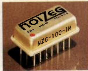
Noise Generators NZG Series/100 Hz to 5 MHz Up to 150 mv output/White Gaussian Noise 14 Pin DIP/Small size and weight Qualified Peak Factor: 5:1 (min) Frequency Flatness: \pm 0.5 DB.
