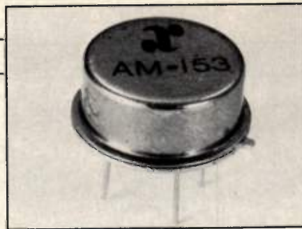
Rather than design an amplifier, engineers have the option of using a broad-band hybrid gain block like this one from the Anzac Division of Adams-Russell.
