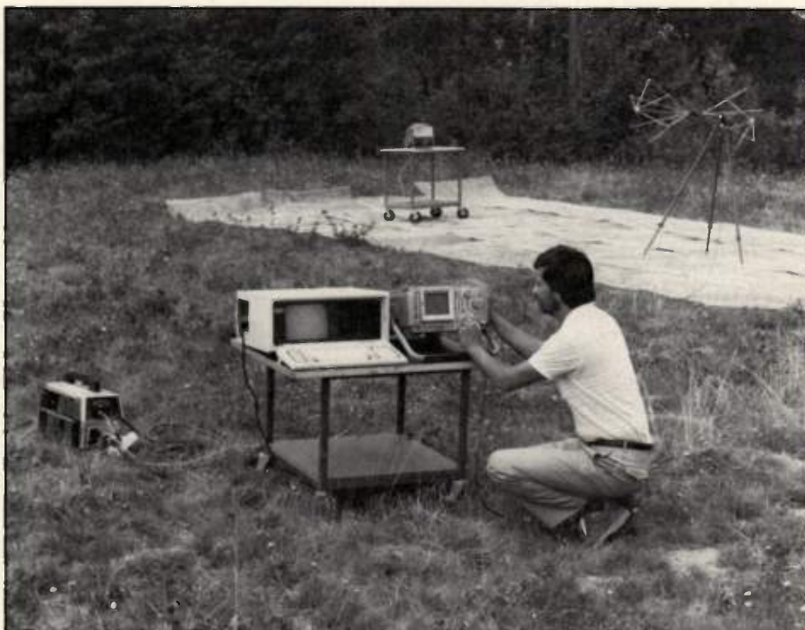
Figure 2. Open-site test system for radiated emissions.
