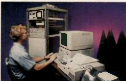
AEMI's HP-8410B Vector Network Analyzer and Sweeper System derives dielectric constants.
