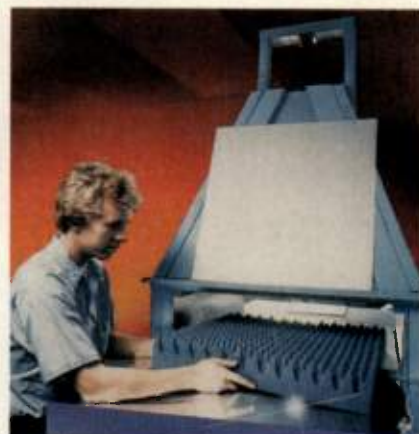
AEMI's transmission tunnel allows measurement of dielectric parameters in the 2 to 18 GHz range.
