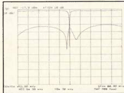
Figure 10. Shows return loss in stopband.
