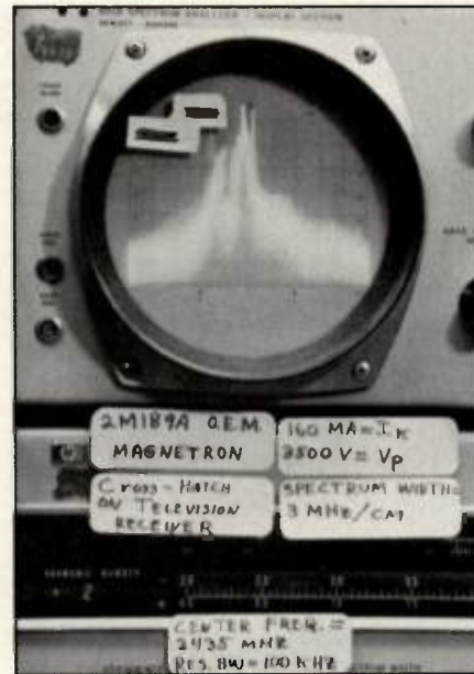
Figure 9. Spectrum display of emitted signal, with cross hatch pattern modulation, 2.5 MHz deviation.
