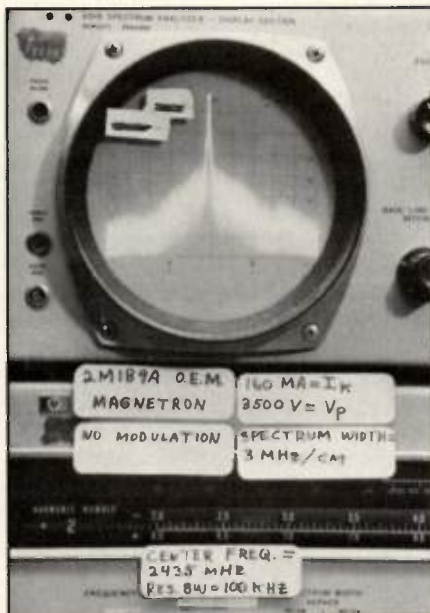
Figure 7. Carrier and noise skirts of unmodulated magnetron.
