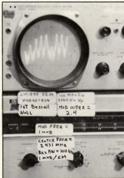
Figure 8. Bessel null display showing primarily FM modulation. I_k variation from + to - deviation is 130-200 mA.
