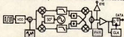
Simulation and lab test of FSK demodulator (block diagram below)
