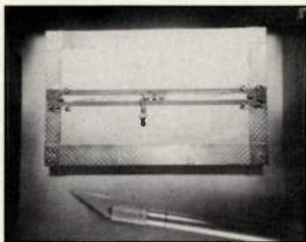
Figure 8. 1.5 GHz MMIC amplifier uses an AvanteK MSA-0285.
