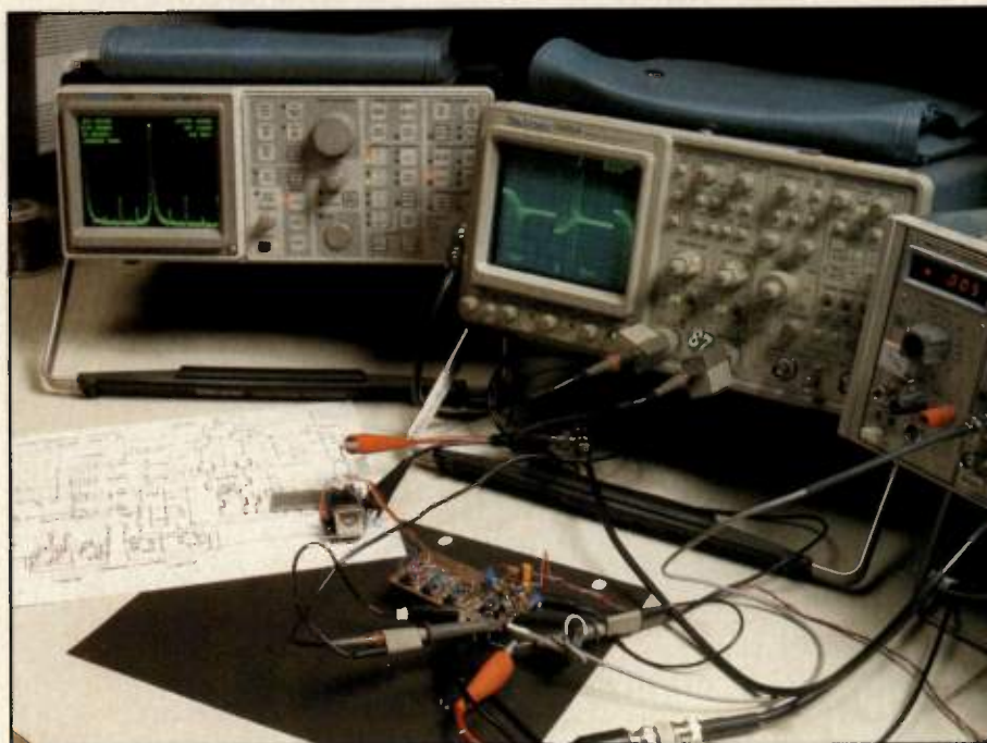
Dan Baker's winning phase detector circuit cancels the reference frequency, reducing the reference sidebands at the output.
