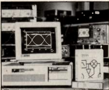
Simulation and lab test of FSK demodulator (block diagram below)
