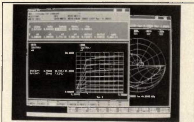
Figure 5. Xtract is used for large-signal and linear model extraction.
