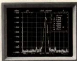
The Receiver Menu for changing the detection mode of the internal AM/FM/SSB receiver or for activating the time shared receiver mode.
