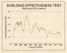
Figure 10. This is a typical plot of shielding effectiveness of an enclosure versus frequency. This technique may be used to evaluate prototype enclosures before the actual product is fully operational.
