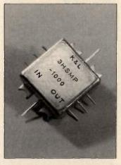
package and has 1.5:1 VSWR and less than 1 dB insertion loss over the 400 to 2000 MHz frequency range. The filter features a cut-off frequency of 200 MHz with a shape factor of 3.0:1 from 3 to 40 dB. Phase matching within ±3 degrees from 400 to 2000 MHz is available. Both units are laser welded for hermetic seals. and both filters are 0.50 inches × 0.50 inches × 0.24 inches (1.27 × 1.27 × 0.60 centimeters) in size. K&L Microwave, Inc. INFO/CARD #209
