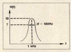
Figure 3. Characteristic graph of H(f) versus f for the circuit shown in Figure 2.
