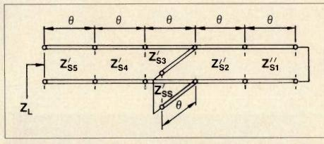
Figure 3. The converted version of the stepped impedance element shown in Figure 1b.
