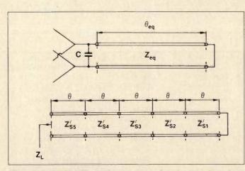
Figure 1. A distributed resonant circuit: (a) electrical scheme of a conventional configuration, (b) five-section stepped impedance element.
