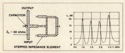
Figure 5. The investigated resonant circuit: (a) microstrip line layout, (b) measured insertion loss function.
