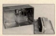
Figure 6. Interior view of the comb generator showing the battery and mounting arrangement.
