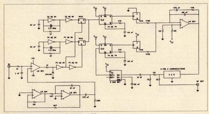
Figure 1. Design example of a linear driftless VCO.
