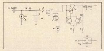
Figure 4a. Schematic diagram of the power supply and battery charging circuit. Ut is an optional voltage regulator used for the 9V battery operated miniature comb generator.
