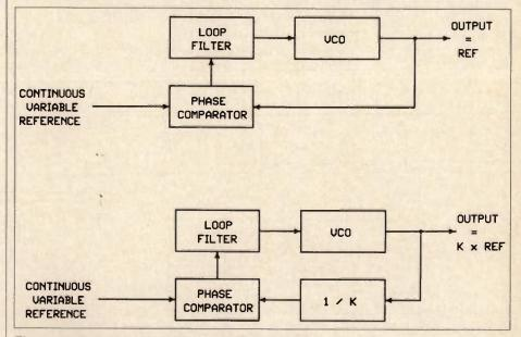
Figure 2. PLL system with an ordinary VCO.
