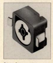
Celsius. Seven capacitance ranges (from 1.7 - 3.0 pF to 13.0 - 50 pF) are available. Each corresponds to the ranges for the J-leaded and top tuning gull-wing models already offered by Sprague-Goodman. The capacitors are 4 × 4.5 × 2.7 mm in size, and prices for Surftrim<sup>R</sup> gull wing trimmer capacitors with reverse leads start at \$0.51 for quantities of 1,000. Sprague-Goodman Electronics, Inc. INFO/CARD #211
