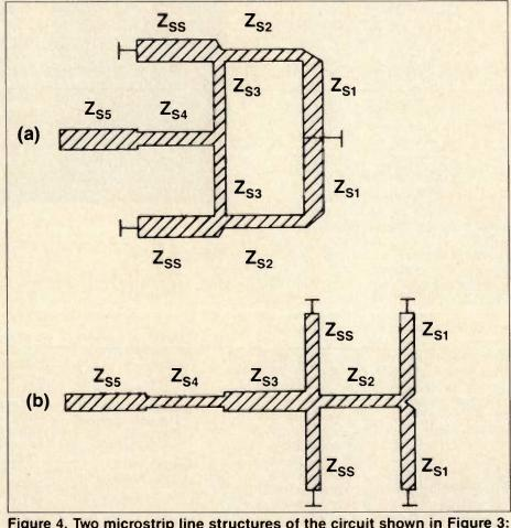
Figure 4. Two microstrip line structures of the circuit shown in Figure 3: (a)  $Z_{S1} = 2Z'_{S1}$ ,  $Z_{S2} = 2Z'_{S2}$ ,  $Z_{S3} = 2Z'_{S3}$ ,  $Z_{S4} = Z'_{S4}$ ,  $Z_{S5} = Z'_{S5}$ , and  $Z_{S5} = 2Z'_{S5}$ . (b)  $Z_{S1} = 2Z'_{S1}$ ,  $Z_{S2} = Z'_{S2}$ ,  $Z_{S3} = Z'_{S3}$ ,  $Z_{S4} = Z'_{S4}$ ,  $Z_{S5} = Z'_{S5}$ , and  $Z_{S5} = 2Z'_{S5}$ .
