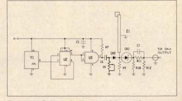
Figure 4b. Schematic diagram of the comb generator circuit.
