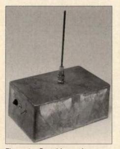
Figure 1a. Portable comb generator with monopole antenna attached.
