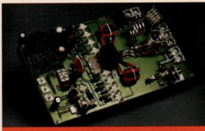
1 KW HIGH EFFICIENCY MOSFET HF POWER SUPPLY, ETO Model SG-1D for plasma and other industrial applications. Available for 13.56, 27.12, or 40.68 MHz, or any frequency 2-41 MHz. RF module shown.
