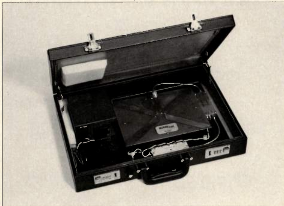
Another use of RF: the portable noise jammer, which makes conference rooms safe for sensitive conversation.
