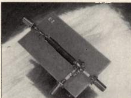
Figure 9. Photo of completed SMT bridge circuit.
