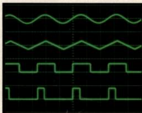
Besides generating precise RF signals, the 6080 Series has a DDS modulation oscillator to generate multiple functions from 0.1 Hz to 200 kHz.
