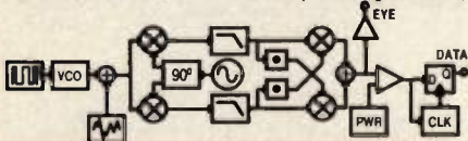
Simulation and lab test of FSK demod (block diagram below)
