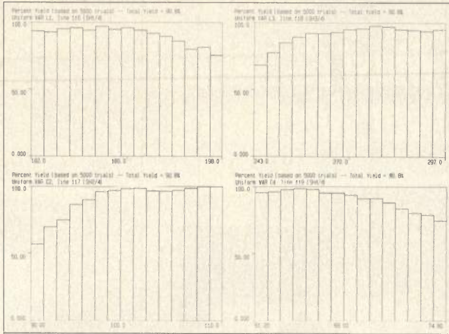
Figure 7. Sensitivity histograms after design centering.
