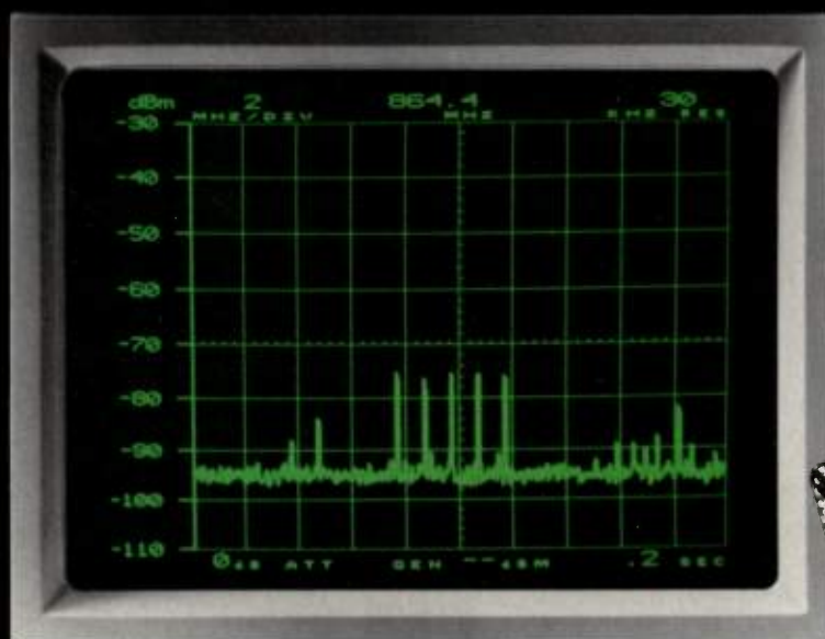
Spectrum analyzer display of cellular telephone transmissions.
