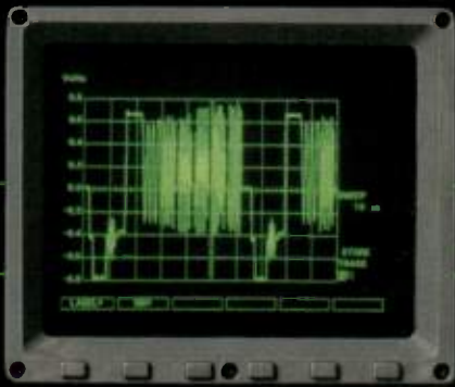
Time domain composite video wave form
