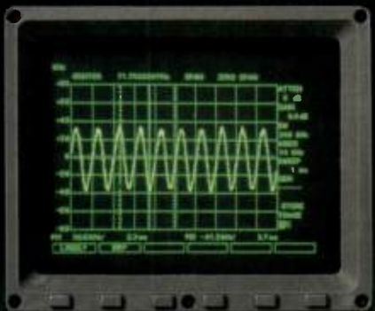
Demodulated FM carrier
