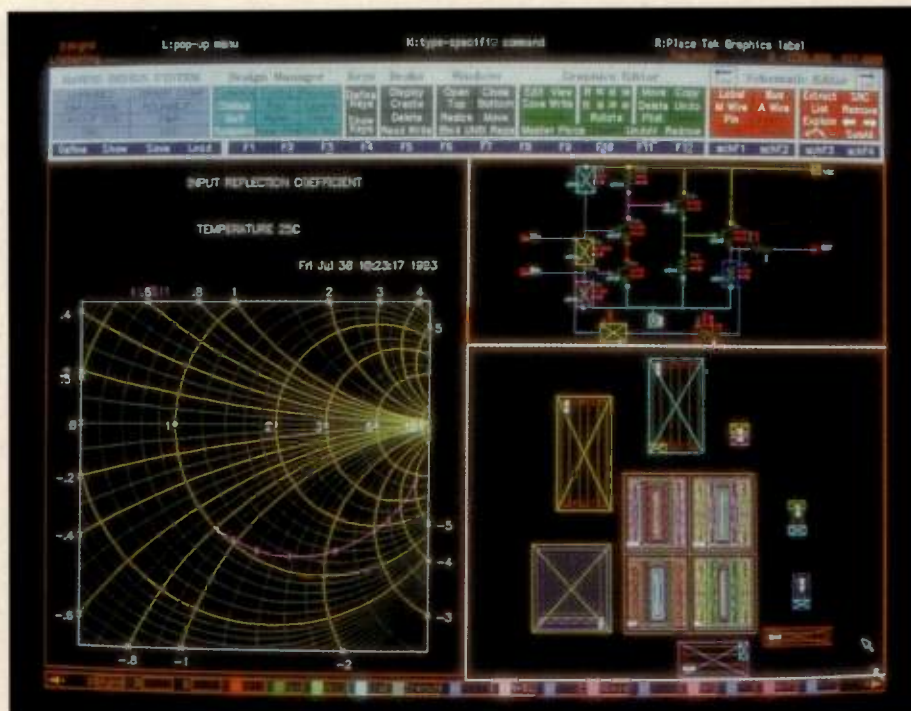
New design tools have the goal of introducing RF-specific design functions into established IC design, layout and simulation systems.
