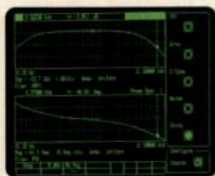
Frequency response - Using the SR770's low distortion synthesized source, Bode plots of amplitude, phase and group delay are quickly generated.
