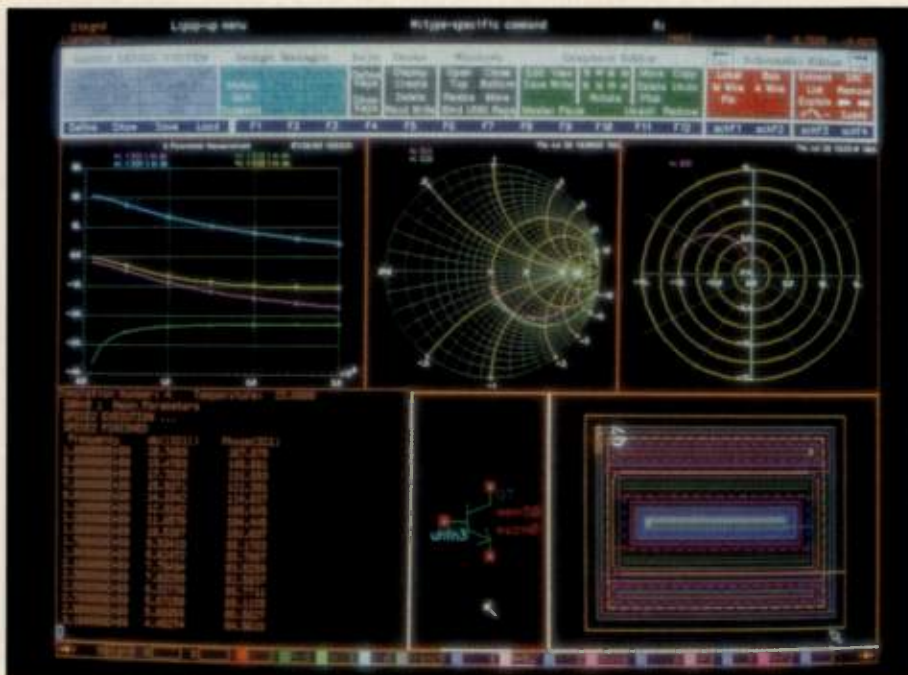
Figure 1. An IC transistor and its auto-synthesized layout. Plots include S parameters in different formats.
