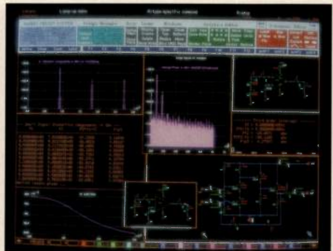
Figure 3. Low noise amplifier, with results of large-signal and small-signal distortion analysis.
