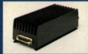
Plug in amplifier for analog cellular 869-894 MHz, 45 Watts
