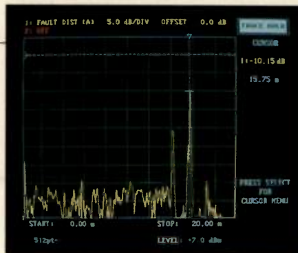
Figure 3: A distance to fault measurement reveals that the second connector is the source of excessive reflection.
