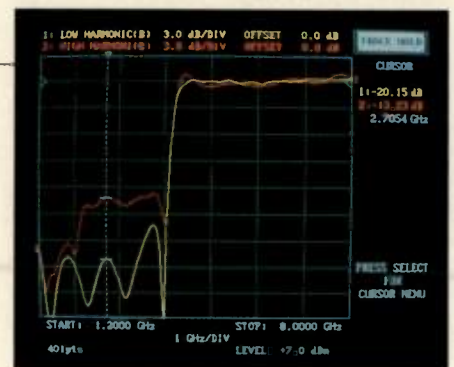
Figure 4: The actual return loss of this low pass filter is grossly distorted by a source's excessive second and third harmonics.
