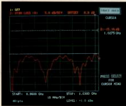
Figure 2: This swept frequency plot of a transmission line cable and antenna marginally meets the -15 dB return loss specification.
