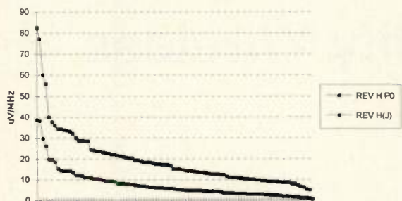
Figure 8. Noise density levels measured at each pin of the engine controller module I/O before and after modifications. Data are sorted from noisiest pin to quietest.
