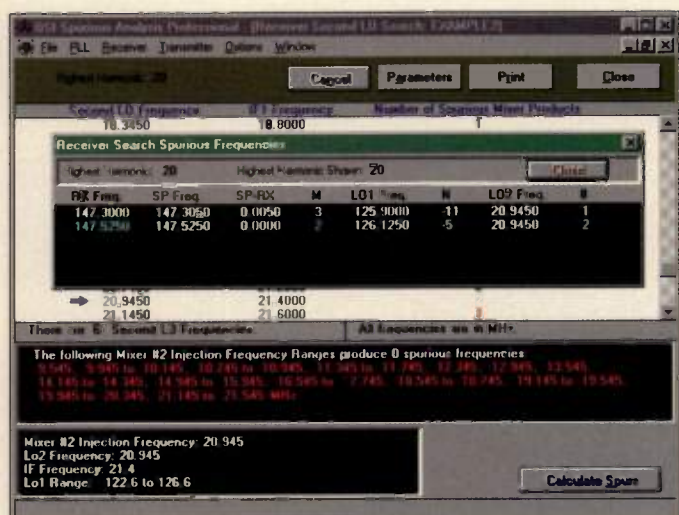
Figure 5. Search table results with "Calculate Spurs" window (Example 2).
