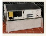
MHz with 0.1 Hz resolution, a frequency switching speed of 20 µs, phase noise of -115 dBc/Hz at 310 MHz with a 1 kHz offset and an output power as high as 13 dBm. Each output channel is controlled through a separate 50-pin parallel interface.
