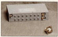
receive isolation typically 60 dB and return loss typically better than 16 dB on all ports. Designed to be used in micro, pico and nano cells, the unit measures  $3'' \times 1'' \times 6''$  and is priced less than \$140 in production volume.
