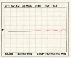
Figure 5. Typical coupled port response.
