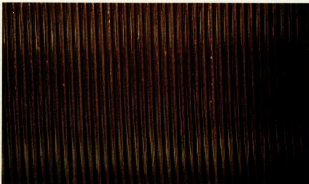
Figure 1. Example of perfectly laid wire due to well implemented quality control.
