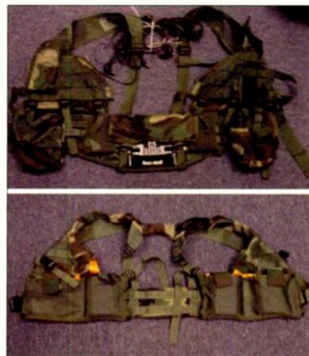
The earlier version of the Land Warrior system (top) had a number of exposed cables. The current version (bottom) is more compact with the use of flex circuitry.
