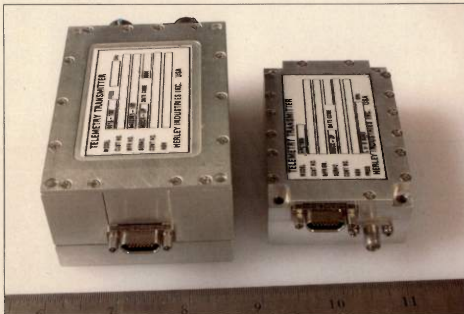
Figure 1: Old 10 W HFQT810, and new HFQT605 5 watt transmitter.
