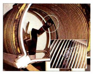
The coil was obviously charred at the tap point. I then powered up the transmitter and checked
