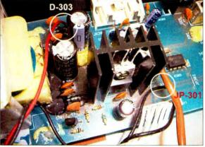
The positive voltage comes from the cathode (banded) lead of diode "D-303, which is located toward the
