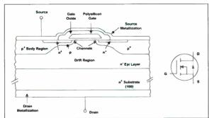
The mechanical and electrical layout of a MOSFET.
