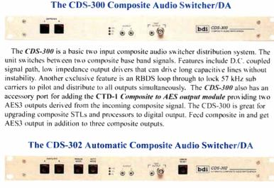
The *CDS-302* is a two input composite audio switcher distribution system with silence sensor for automatic switchover operations. The *CDS-302* has all of the features of the *CDS-300* above including accessory port for adding the *CTD-1 Composite to AES output module*. Provides complete confidence that audio will get to the transmitter in the event of a link failure.
