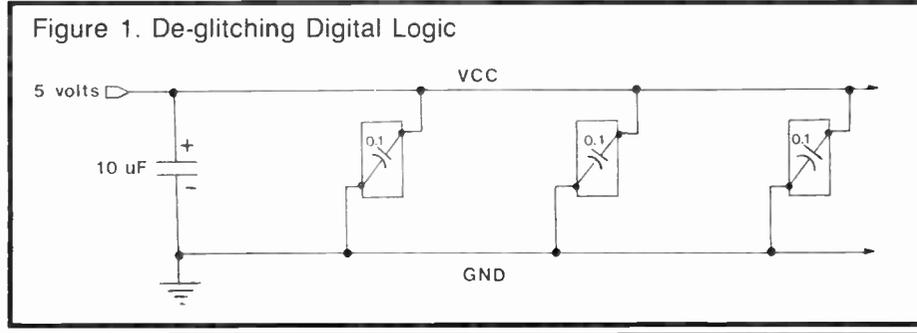
the audio circuits, but digital will just glitch when the crosstalk signal peaks above the logic threshold.
