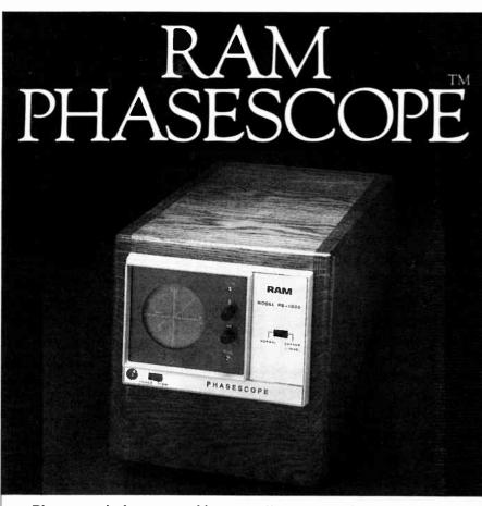
Phasescope is the new word in economical-visual stereo monitoring. The Phasescope is priced to be affordable for every control room and studio. It displays the classical stereo starburst when monitoring stereo audio or a straight line when a mono signal is present. Designed with the operator in mind, the Phasescope contains a minimum of
