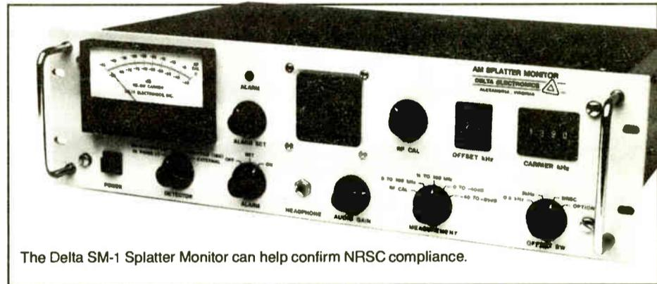
The Delta SM-1 Splatter Monitor can help confirm NRSC compliance.
