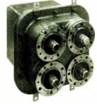
Coaxial Transfer Switches—These 1 %" and 31/8" motorized four port switches are designed to switch between antennas, transmitters, or dummy loads both quickly and efficiently. The switches can also be operated manually and are fully interlocked.
