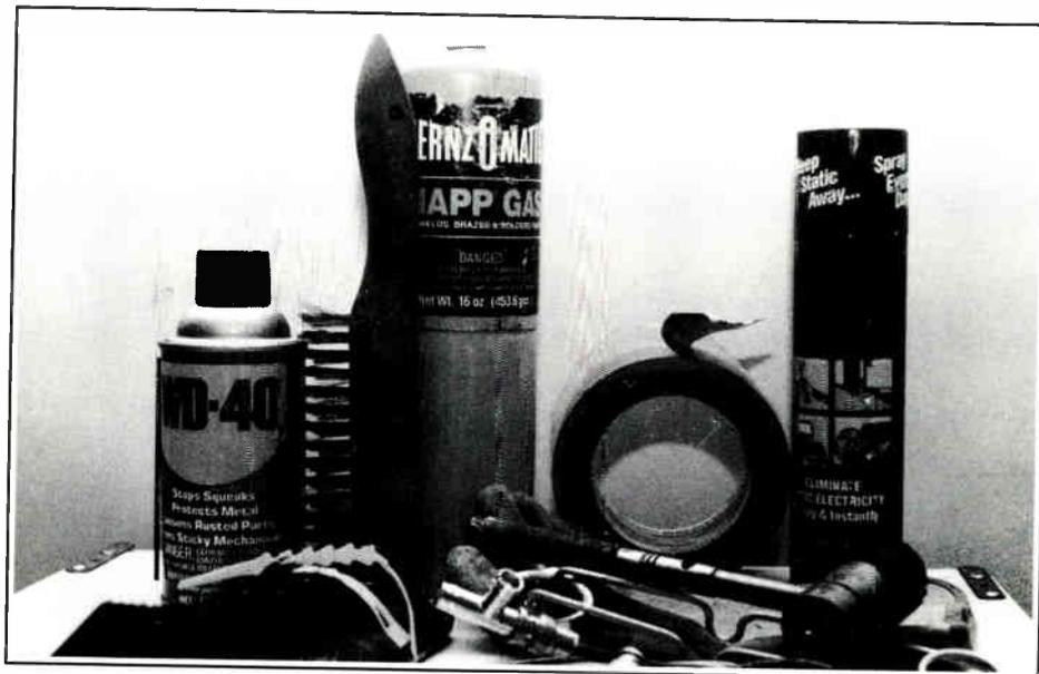
A trash bag for your dish, MAPP Gas for quicker silver solder connections, WD-40 for removing duct tape residue, and Static Guard for your studios. Just a few of the items to speed your job.
