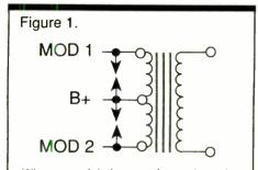
When a modulation transformer loses its safety gaps, it fails to dissipate transient energy that might cause damage.
