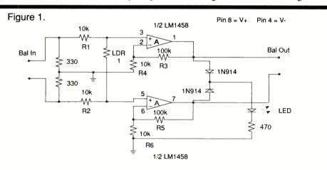
nal. When the balanced signal is reduced, each op-amp receives less signal, and, a reduced output is reflected.
