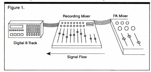
month later. We considered two different ways to record the concert: Either split the mics to feed both the P.A. mixer and the recording mixer or take direct-outs and group-outs from the PA mixer into the recording mixer.
