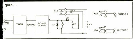
t connect a timer and relay together. e normally open (N.O.) contacts uld operate the On/Raise function of a nsmitter and the normally closed .C.) contacts would handle the f/Lower inputs. This is not a good a, as it is comparable to someone ding their finger on the Up or Down tton continuously after the control nmand had taken place.
