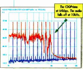
On just one of the two digital channels of an ISDN circuit, Zephyr's Layer III delivers 15kHz mono audio.
