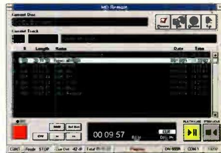
Denon's MD Remote™ Software, running under Windows™, offers a graphical interface for fast, easy control of all functions and modes on any Denon MD Cart machine, including automatic dubbing of tracks or discs between machines, complete with titles and cue-point information.
