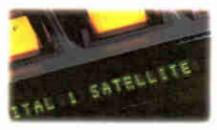
Each fader bas a 10-character alphanimeric display. The display changes when another andio source is assigned, which can happen either manually or at a preassigned time.
