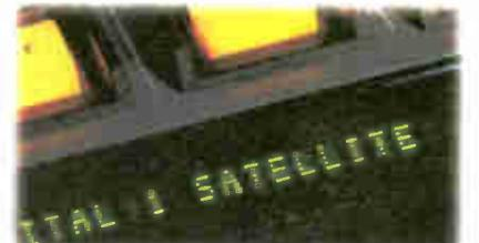
*Each fader has a 10-character alphanumeric display. The display changes when another audio source is assigned, which can happen either manually or at a preassigned time.*
