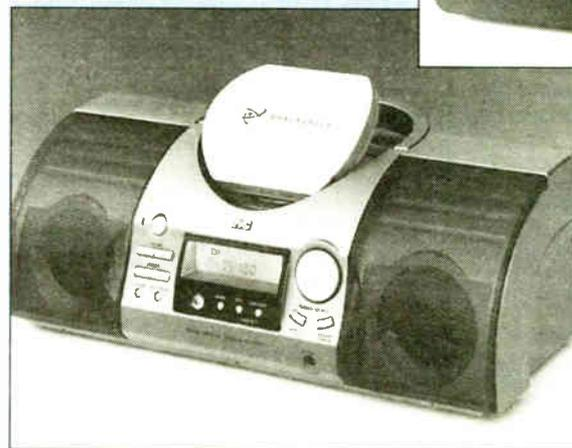
The JVC FR-DS100 (left) and Hitachi KH-WS1 (top) include FM, mediumwave and shortwave reception capabilities alongside L-band reception.
