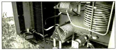
Figure 4: Clean out the inside of the coupling unit.
