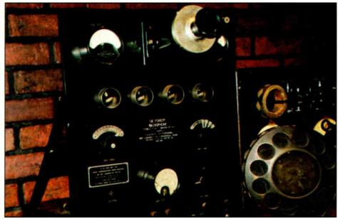
Equipment for WWJ(AM) in Detroit dates to 1920 when the station signed on the air as 8MK. Featured are a De Forest T10 Radio Phone and De Forest R-800 Combination Audion-Ultraudion Detractor and One Step Amplifier which served as console and amplifier.
