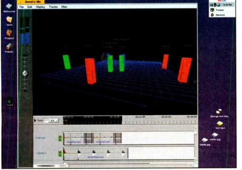
In the 3D mode, individual tracks are represented spatially. Tracks are dragged left and right to control placement, and front to back to control volume.
