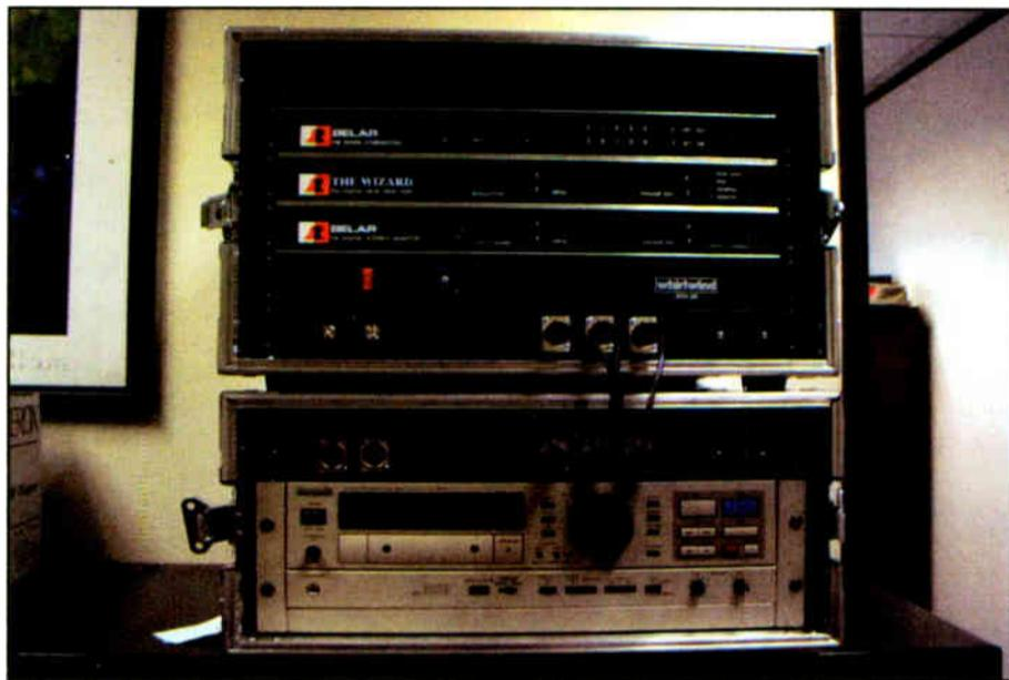
Packaged as two rack cases by Radio Systems, the Belar Wizard Mod Monitor and DAT for sample collection are a manageable set. Components can be used together or individually.
